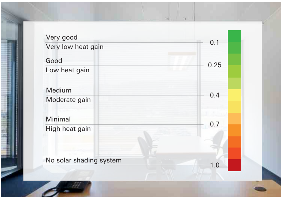
Graphic for 1.–3.: Solar shading Characteristic values for reduction factors F_c of external shading systems.
